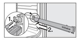
■ Fit the telescopic runner in between the two rails at the front (1) and then push it into the oven compartment (2).
